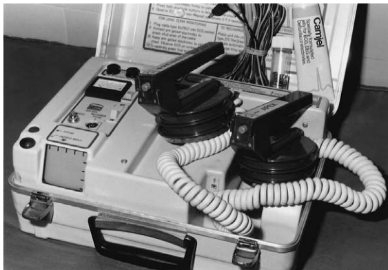
FIG. 20.7 Defibrillator for external use. For reasons of safety in use both the electrodes have switches in their insulated handles. These switches need to be pressed simultaneously to deliver the shock. This particular model of defibrillator has its own monitor ECG.
