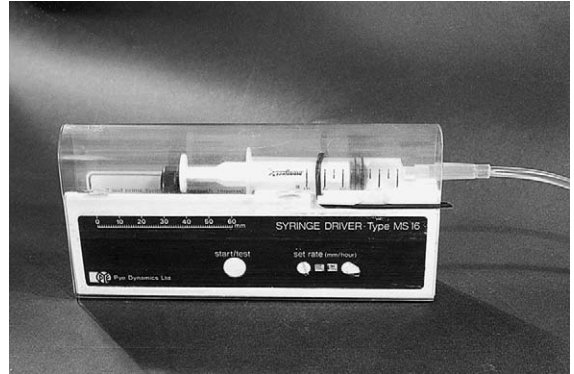
FIG. 9.5 Syringe driver. Many types of electrically driven syringe drivers are available. Some must be used with one specified size of syringe, others can be used with a variety of syringes.
