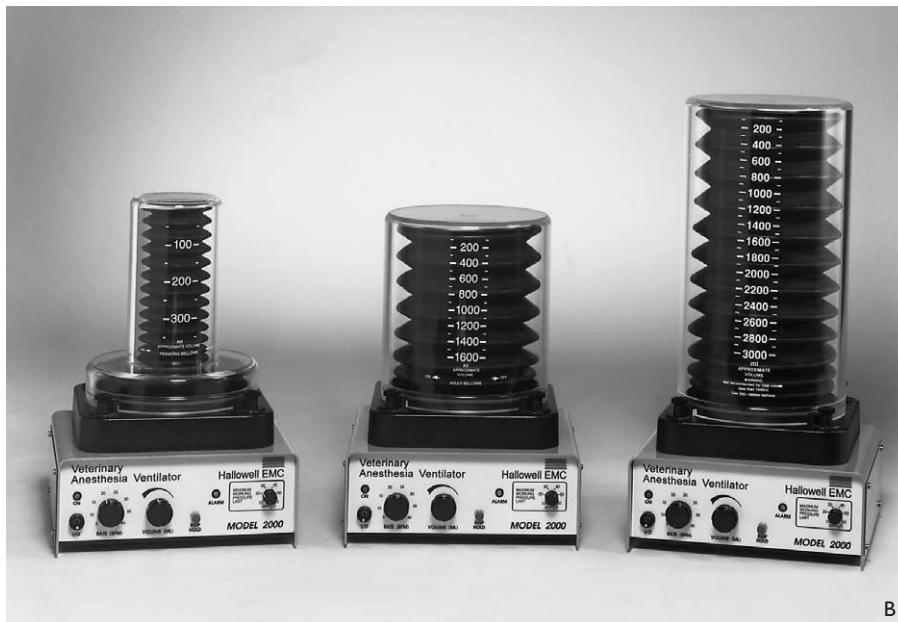
FIG. 8.8 A, B One example of a ventilator specially designed for veterinary use is the Hallowell ventilator, which is widely used in North America and elsewhere. It is electronically controlled, time-cycled and pressure-limited. Interchangeable bellows and housings enable it to deliver accurate tidal volumes of from 20 ml to 3000 ml at safe working pressures of 10–60 cm H 2 O with respiratory rates of 6–40 breaths per minute. It can be fitted to all anaesthesia systems with out-of-circuit vaporizers (photographs courtesy of Hallowell EMC, 63 Eagle Street, Pittsfield, Massachusetts 01201, USA).
